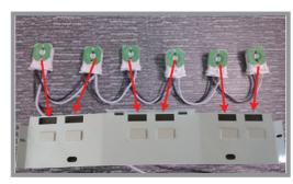
8. Screw socket panel back on. Only one set of sockets will be replaced. The other sockets are now just mechanical holders for the tube. Replace the other side sockets if necessary.
