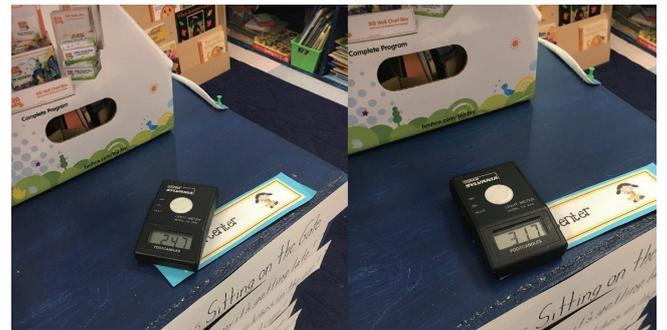
The average light level increased by 28% and immediately saved 60% on energy costs. The issue of color temperature was solved by Starco 4000K LED T8 lamps. The fixtures will not turn yellow, thanks to Starco's unique plastic technology. Due to the long lasting LEDs and LED drivers, the maintenance attributed to lighting will be reduced as well. Finally, in the future, it will be very simple to replace the LED lamps in the fixtures.
