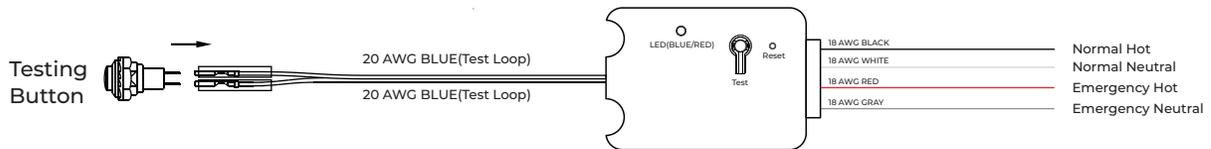
The IFS101 Sensor/Load Controller can be set to emergency mode (IFS101E) by default raising the light levels to 100%. It only allows sensor control and dimming when an active signal from the PPA109S is signaling that normal power restored. Standard operation of the IFS101 requires a wireless signal from the PPA109S that normal power is lost to go into emergency mode, bypass dimming and control functions.
